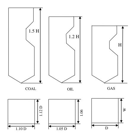
The figure above illustrates the relative size of units designed for these three fuels.
